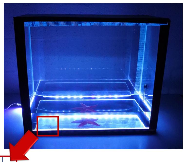
Experimental aquarium equipped with a total internal reflection (TIRF) system (highlight)
