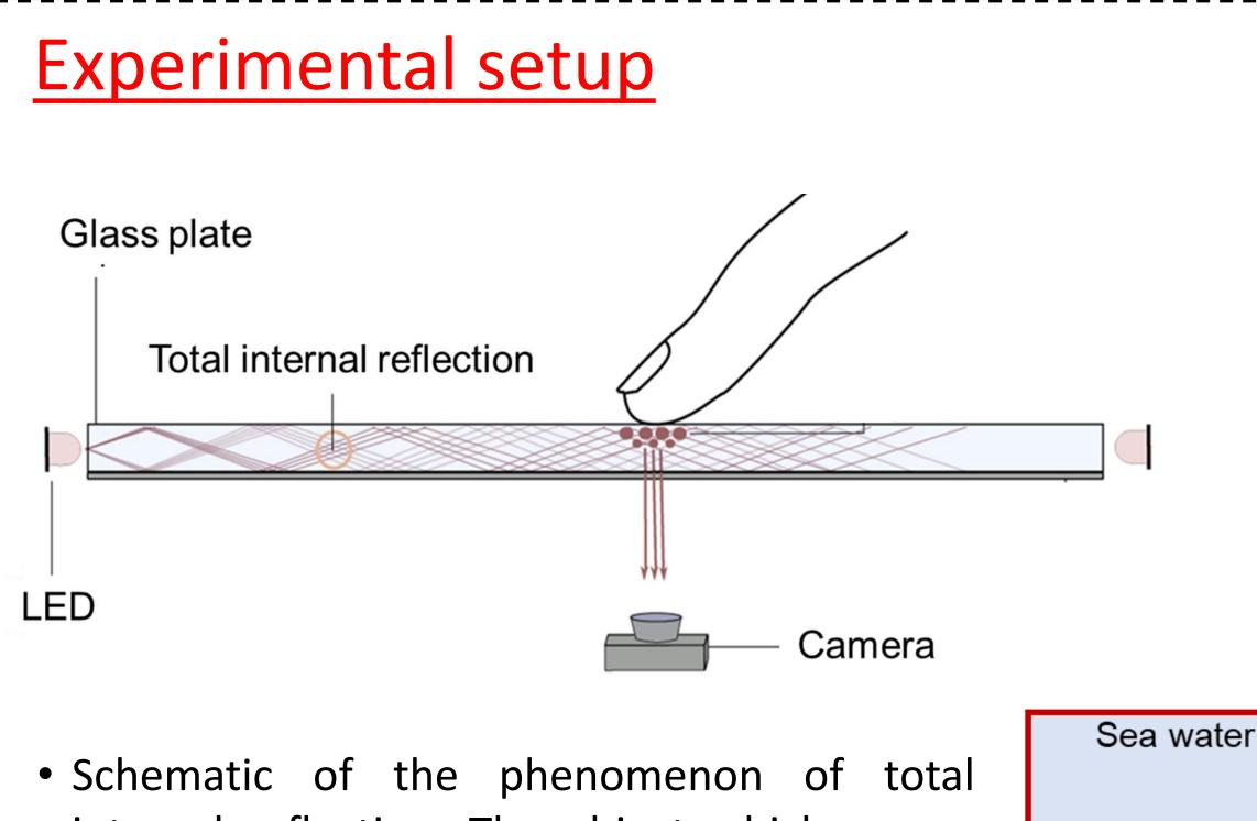
internal reflection. The object which comes into contact with a surface provided with the TIRF will diffuse the light and this contact area will be illuminated.
